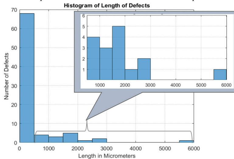
Figure 2. Histogram of Defects Detected from Image in Figure 1
