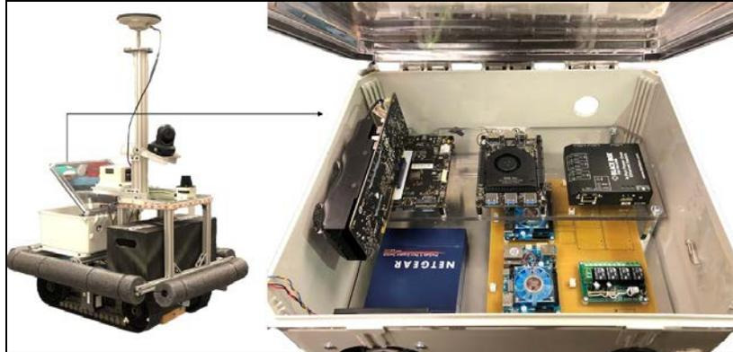
Figure 1. Intelligent Vehicle of Autonomous Navigation (IVAN) and an enlargement of the Computing System
