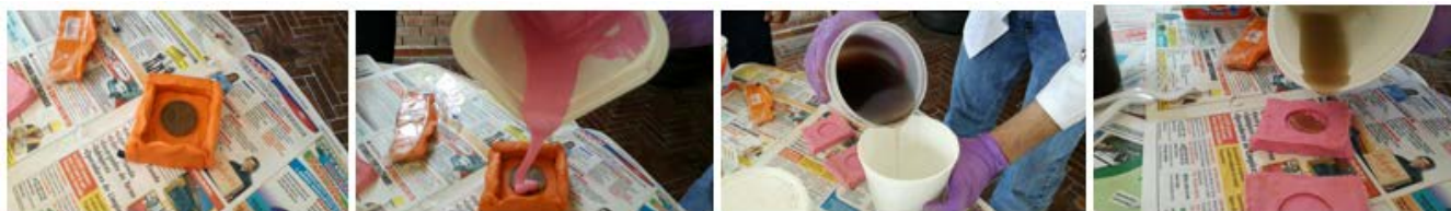
Figure 2. Experimental process of elaboration, in the first photograph you can see the placement of the study object in the mold, in the second the emptying of the rubber silicone, in the third the creation of the resin, and finally the emptying of the resin in the rubber silicone mold.
