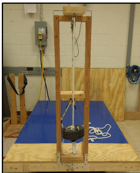
Figure 1. Custom-built wooden structure to support hanging weight
