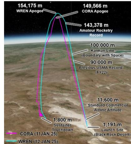
Figure 7: CORA and WREN Vehicle Flight Path
