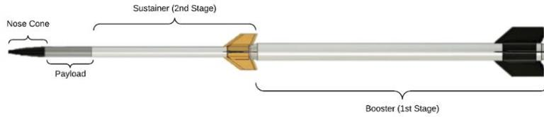
Figure 6: CORA and WREN Vehicle Architecture
