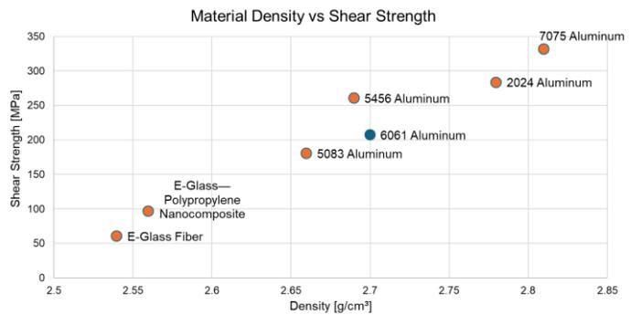
Figure 3: Material Density vs Shear Strength Tradespace
