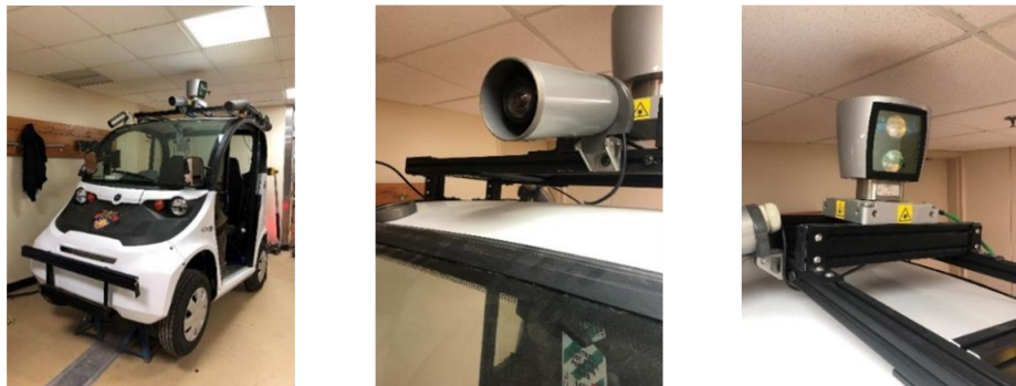
Figure 1. Polaris GEM E2 with LiDAR and Mako Cameras Left to Right: Polaris GEM, Mako Camera, LiDAR
