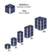
Figure 1. CubeSat Sizes and Configuration
