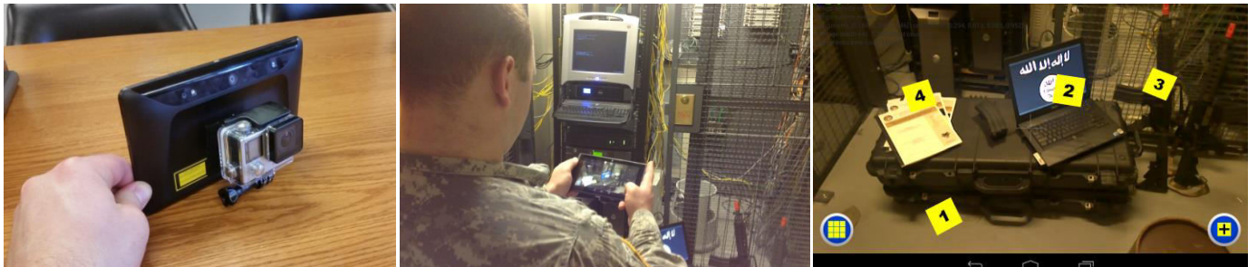
Figure 1. The Raven Eye system (left) is used by a soldier (center) to exploit a sensitive site. A screen capture from the system (right) shows tracked, virtual tags (yellow numbers) which annotate and geo-locate items of interest as the soldier navigates the scene.
